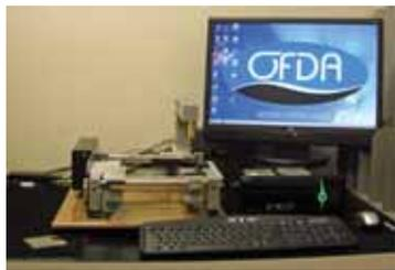
*Laboratory bench model operated under standard conditions under standard conditions for testing textiles, 20°C, and 65% relative humidity (+2% RH). This OFDA2000 operates on staple profile or OFDA100 mode.*
