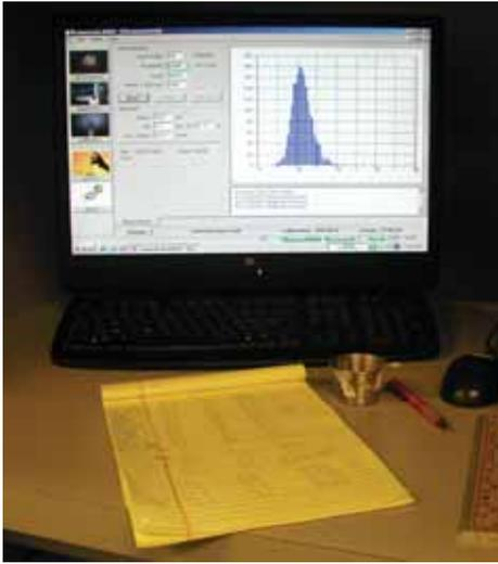
**Histogram display on computer screen of fiber measurements recorded by SIROLAN Laser Scan**
