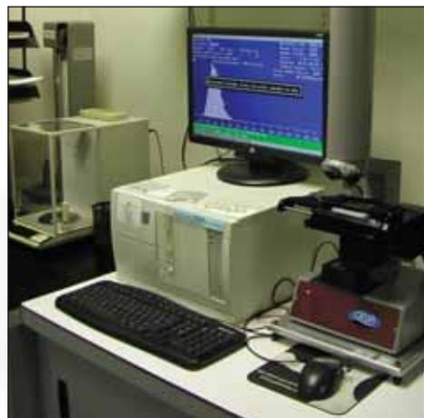
**OFDA100 software analyzes fiber images and derives MFD, SD, and CV measurement of 2000 to 4000 longitudinal fiber sections. OFDA100 also**
